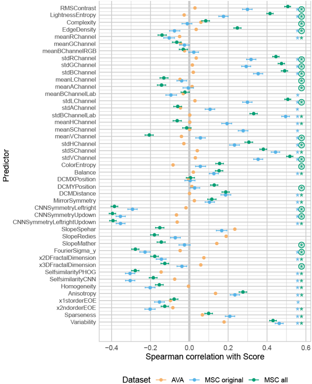
Figure 7: Regression analysis across the three databases using all metrics from the QIP toolbox 44 . We computed Spearman rank correlations between aesthetic scores and 45 image metrics from the QIP toolbox for each database (AVA, orange; MSC original, light blue; MSC all, green) using a bootstrapping procedure. Each row corresponds to a different metric. The 95% confidence intervals for the correlation coefficients are shown in the color of the corresponding database. (For AVA, the intervals are extremely narrow due to its large sample size and are therefore not visible.) Colored markers on the right indicate statistically significant differences in correlation strength between databases: blue stars mark cases where the correlation for MSC original is significantly greater than for AVA; green stars indicate where MSC all shows a significantly greater correlation than AVA; and green circles show where MSC all has a significantly greater correlation than MSC original. These results support the conclusion that using a database with a more uniform distribution of aesthetic valuations enhances the ability to detect, and accurately quantify, relationships between low-level image metrics and aesthetic valuation.
